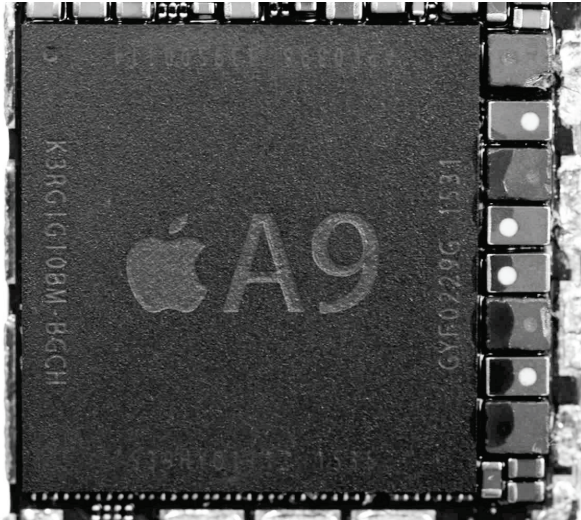
Image 4-4: Apple A9 chip, courtesy AnandTech and iFixit
