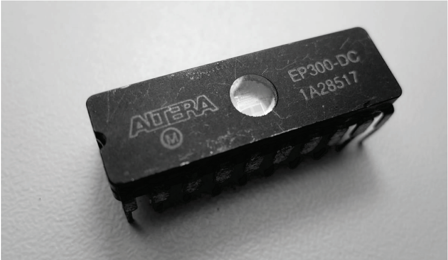
Image I-3: Altera EP300 programmable logic device
