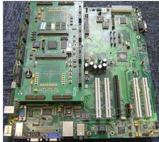
Figure 2. FPGA platform of Godson-2G
