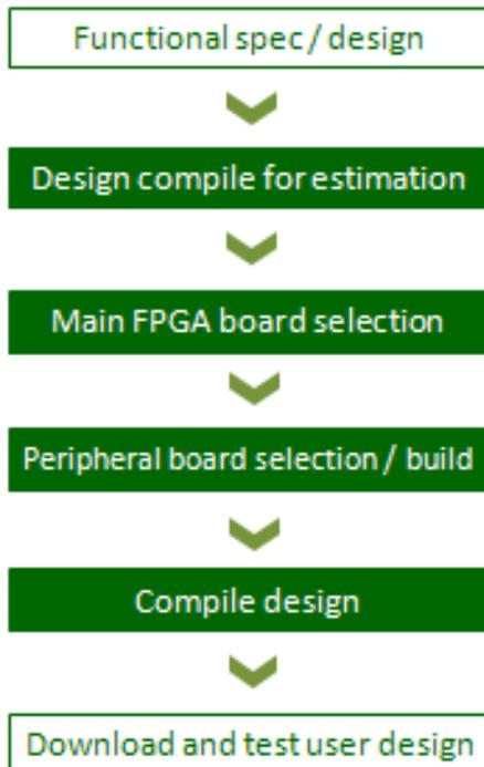
A commercial board solution eliminates several auxiliary steps in the FPGA prototyping process, potentially saving one to three months of design time for the average (12-16 month?) project.
