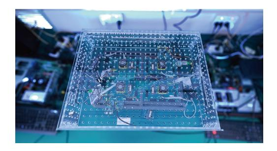
S2C prototyping solution included a diverse selection of daughter cards such as PCIe, HDMI, DDR, and GPIO that made it incredibly convenient to build a GPU verification system. Our client opted for S2C's Prodigy Virtex UltraScale VU440 Logic Systems, which consisted of one Quad platform and one Dual platform, and achieved an impressive FPGA utilization rate of 71%.
